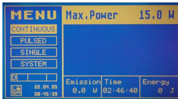
Fig. 20: Parameter menu after switch on the laser system (Power setting 15 W)
