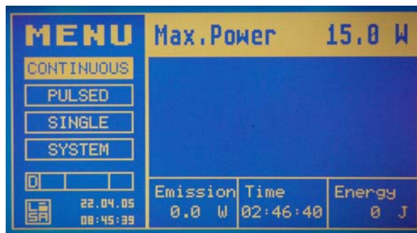
Fig. 22: Parameter menu for continuous mode
