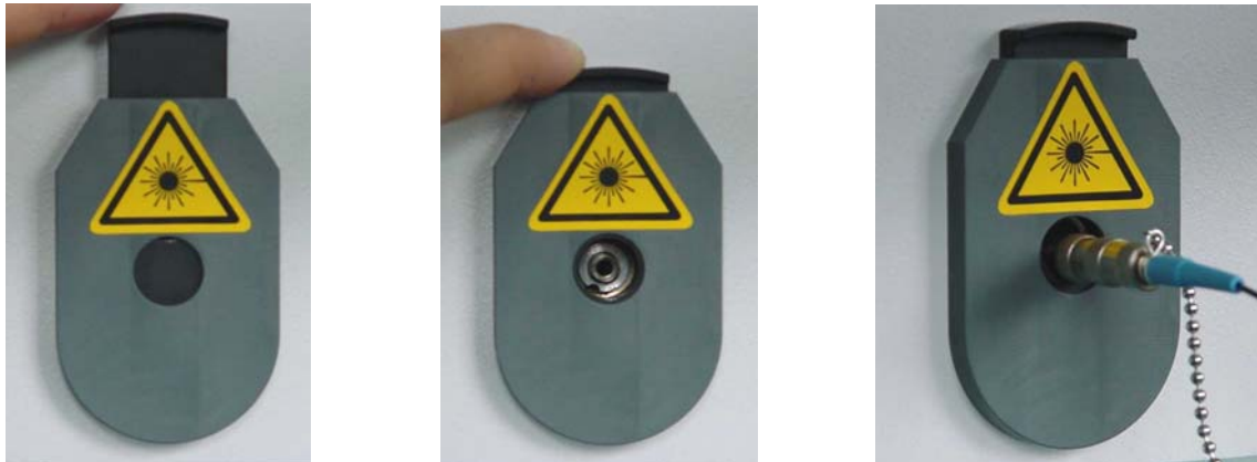
Fig. 18: Connecting the fiber
